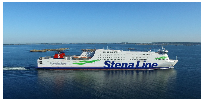
Figure 7. The Stena Germanica , a ferry converted to operate on methanol fuel (photo courtesy of Stena Line).
